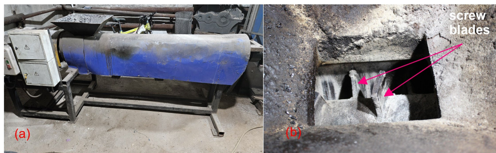
Figure 4. General view of extruder (a) and special design screw (b).
