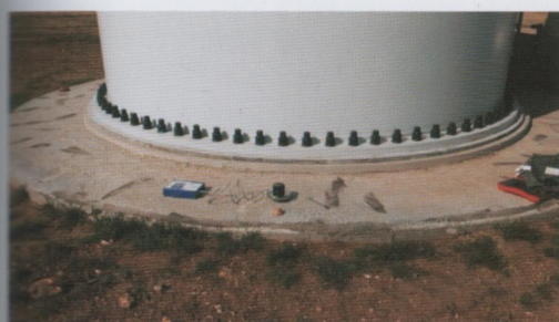
Figure 5 – Fixing a vibration indicator on WPU foundation
