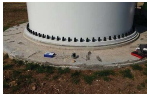
FIGURE 3. Installation of a vibration sensor on the WPP foundation
