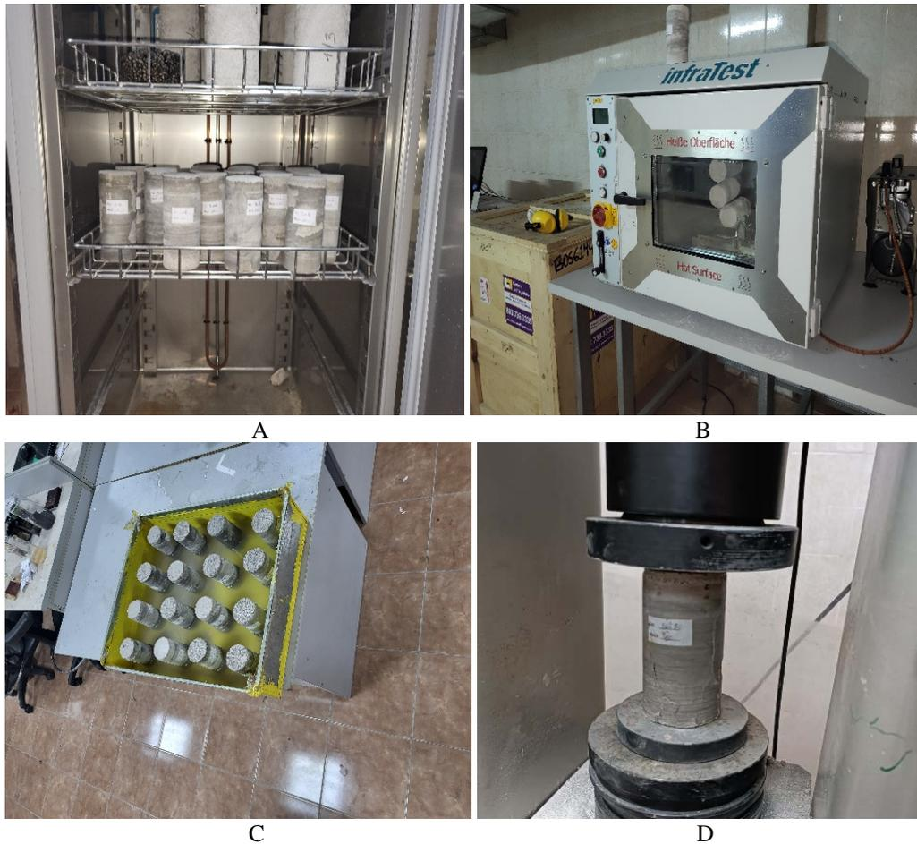
Fig. 2 Testing of foam concrete samples
