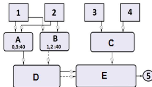
A - container for low-concentrated solution of plasticizing foam concentrate additive in water 0.23:85; B - container for solution of modified foam concentrate in water 1.2:40; C - cement-sand mixer; D - foam generator; E - mortar mixer;  $\odot$  - dosing unit;  $\longrightarrow$  - primary foam injection;  $-\ - \longrightarrow$  - secondary foam injection.
