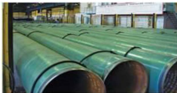
Figure 3 – Pipes with factory polypropylene coating
