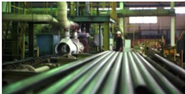
Figure 6 – Pipes with glass-enamel coating
