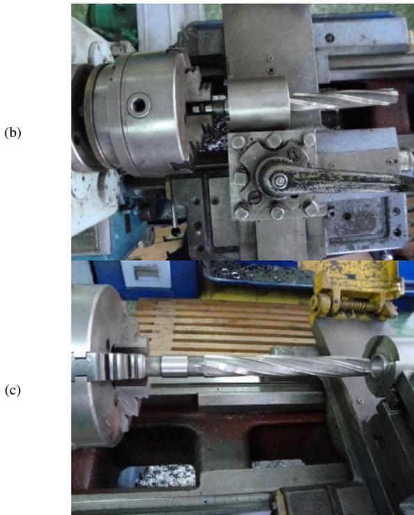
Fig. 5. Scheme of processing a hole using a reamer-broach: (a) processing scheme, where: 1. reamer-broach, 2. workpiece, 3. device housing, 4. jig, (b) starting position, (c) ending position.
