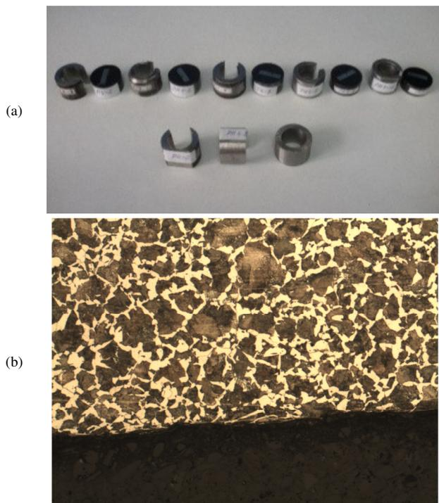
Fig. 11. Results of the microstructure of the surface of holes processed by a reamer-broach.
