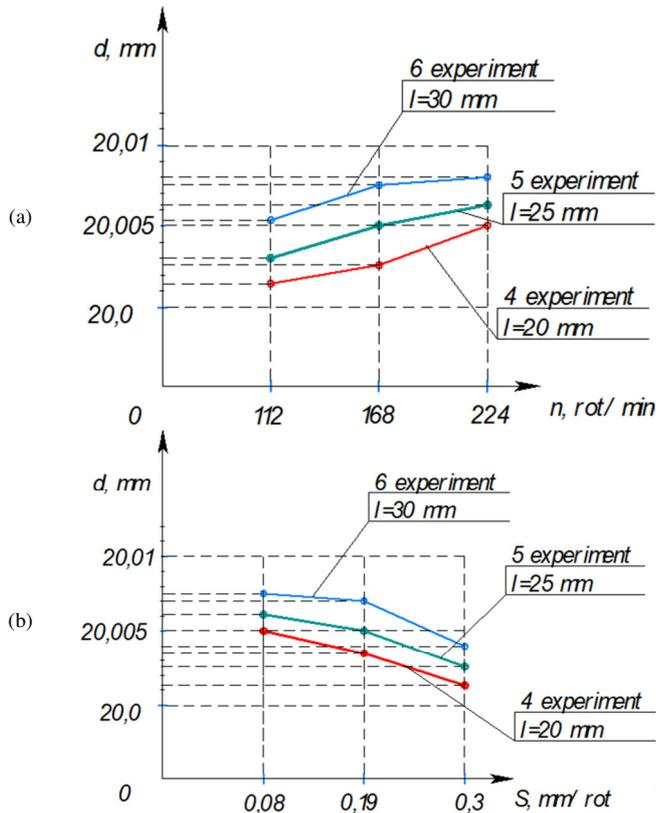
Fig. 9. Dependence of diametrical dimensions on: (a) rotational frequency, and (b) feed.
