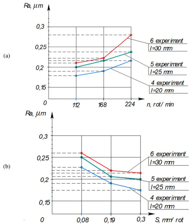
Fig. 10. Dependence of the surface roughness on: (a) rotational frequency, and (b) feed.
