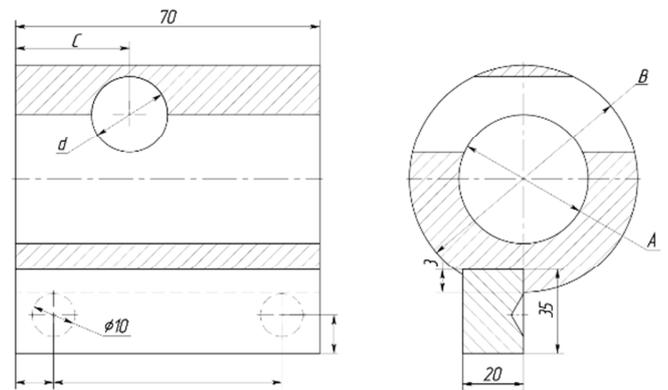
Fig. 6. Device for securing the reamer-broach in the tool holder of the machine support. A: the inner diameter of fixture, B: the outer diameter of the fixture, C: the distance to the axis of the pin, and d: the outer diameter of the pin.
