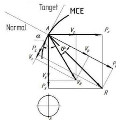
Fig. 4. Forces and velocities during machining.
