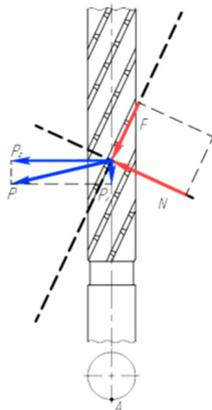
Fig. 2. Cutting forces during machining.
