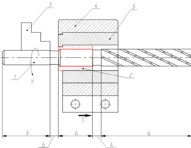
Fig. 7. Installation of workpiece in fixture. 1. reamer-broach, 2. workpiece, 3. jig, 4. device housing, 5. insert,  $V$  is the cutting speed,  $S$  is the supply,  $l_1$  is the front shank length,  $l_2$  is the neck length,  $l_3$  is the front guide length,  $l_4$  is the length of the annular groove, and  $l_5$  is the length of the cutting part.
