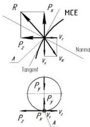
Fig. 3. Technological cutting forces and velocities during machining.
