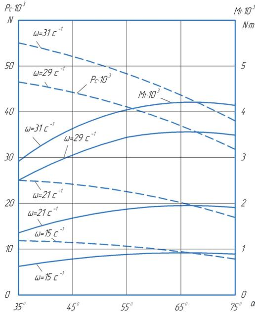
**Fig. 5.** Graph of changes in centrifugal force and torque depending on the angle of rotation of the half-couplings.
