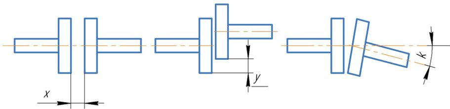
**Fig. 3.** Displacement of shaft axes.
