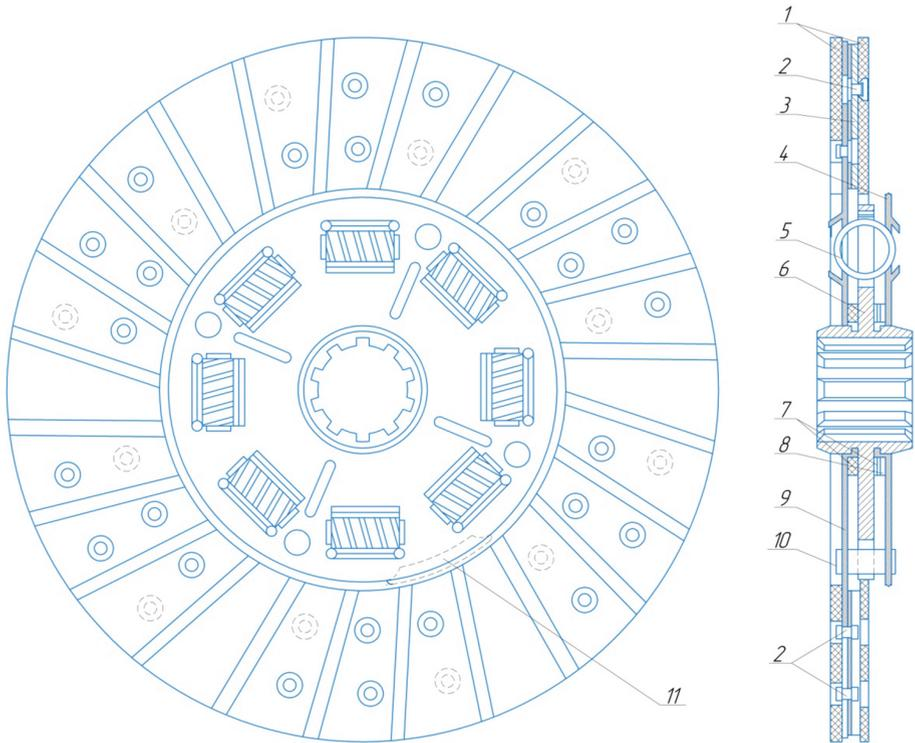
**Fig. 1.** Driven clutch disc: 1-friction pads, 2-rivets, 3-spring of the driven disc, 4-damper plate, 5-damper spring, 6-hub, 7-friction rings, 8-adjusting rings, 9-driven disc, 10-thrust pin, 11-balancing weight.
