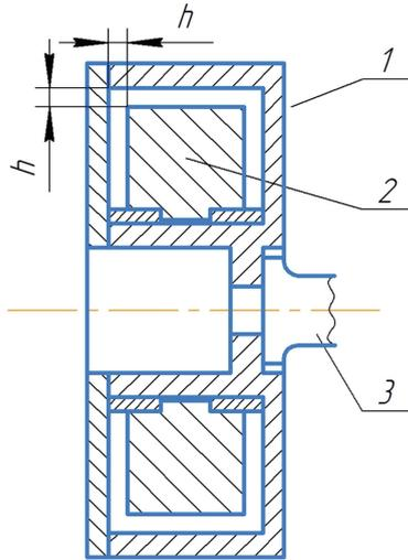
**Fig. 2.** Silicone damper: 1-housing, 2-flywheel, 3-crankshaft
