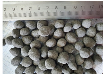
Fig. 1. General view of a bulk granular filter
