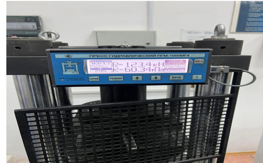
Figure 3 – Results of measuring the fracture force of cast iron casting
