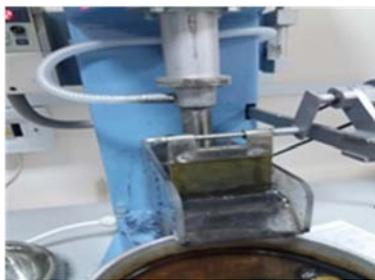
Fig. 1. Flotation machine “Mekhanobr Tekhnika”
