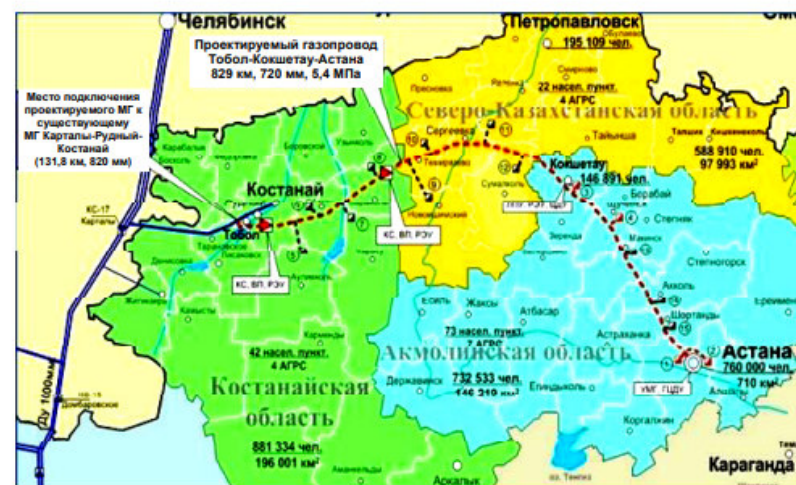
Figure 3 – The Tobol-Kokshetau-Astana gas pipeline [16]
