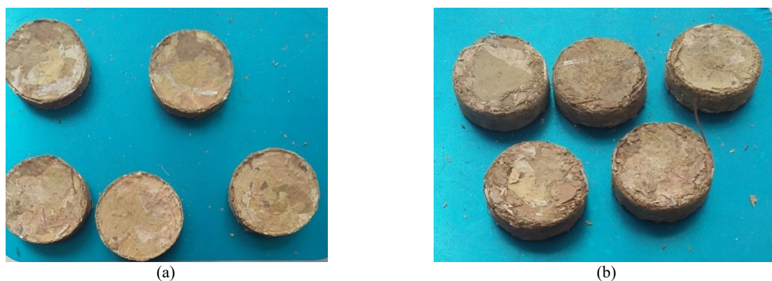
FIGURE 2. Samples of briquettes from non-crushed leaves: (a) – before strength measurement, (b) – after strength measurement.
