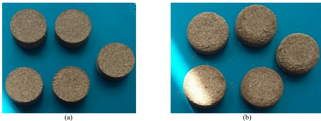
FIGURE 1. Samples of briquettes from 0.2 to 1 mm fraction: (a) - before strength measurement, (b) - after strength measurement.
