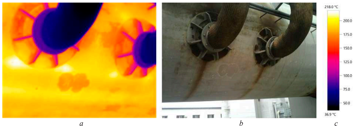
Fig. 2. Zones of elevated temperatures in the tuyere area: a – thermal image of the outer surface of the calcination furnace; b – area of the surface of the calcination furnace; c – temperature scale of the thermal imaging image
