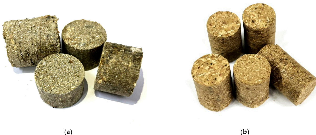
Figure 1. Briquettes from organic and industrial residues. (a) 70% sunflower husks and 30% coke breeze; (b) 30% sunflower husks and 70% leaves.
