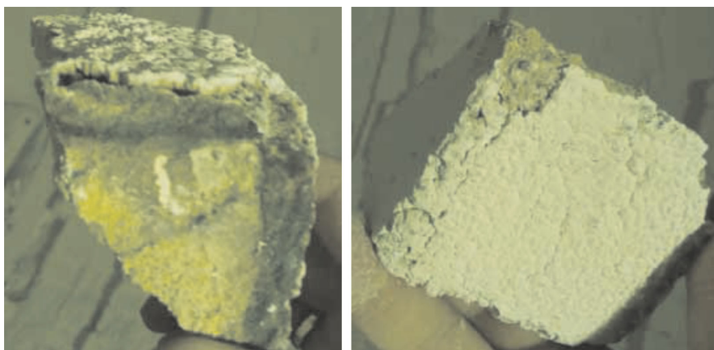
Fig. 2. Chamotte refractory impregnation from calcination zone.
