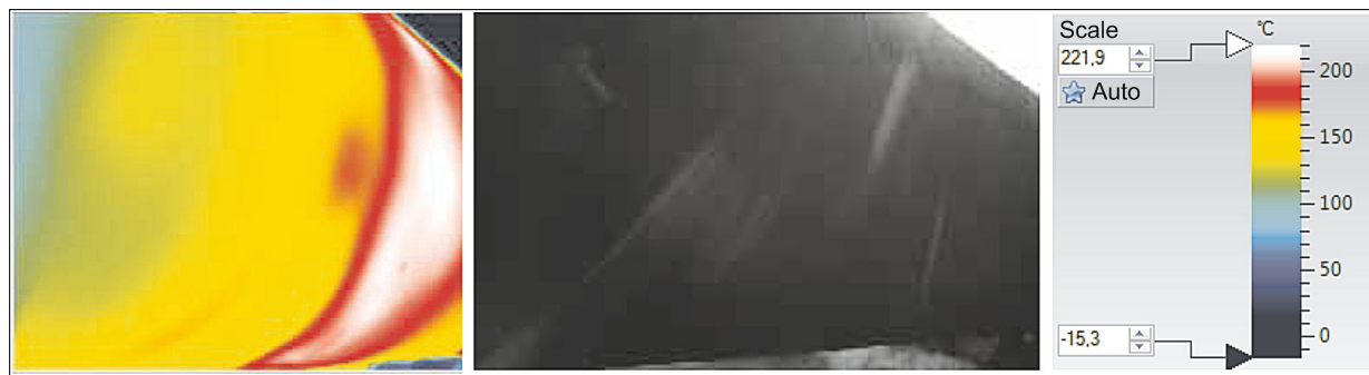
Fig. 1. Start of the calcination zone in a thermogram.
