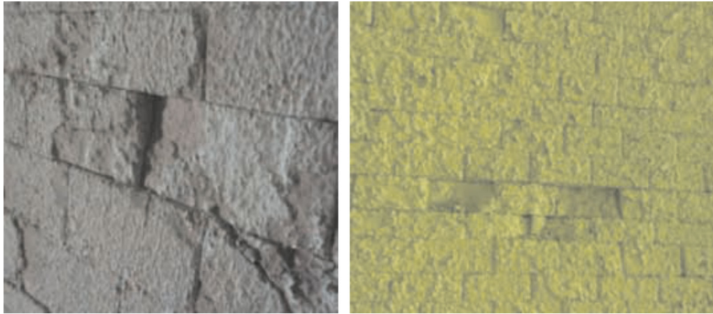
Fig. 3. Calcination zone lining after rotary furnace service.
