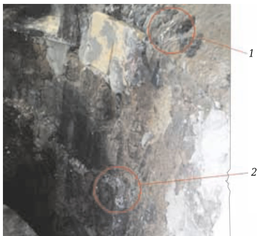
Fig. 5. Pouring ladle lining after three melts: 1) coated by solidified metal; 2) coated by solidified slag.
