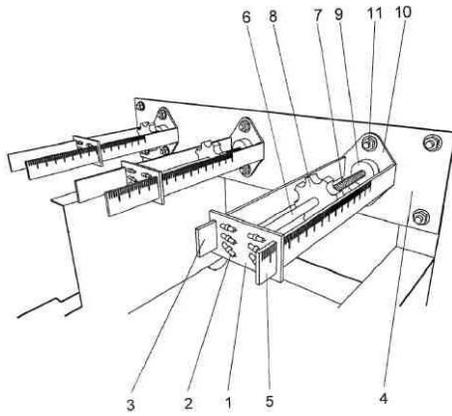
Fig. 1. Measuring device of protection circuit mounted in the compartments of cubicle switchboard (general layout) (part 1)
