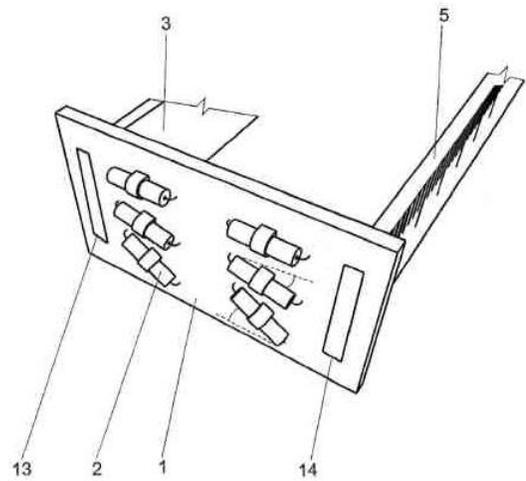
Fig. 4. Layout of a plate with reed switches
