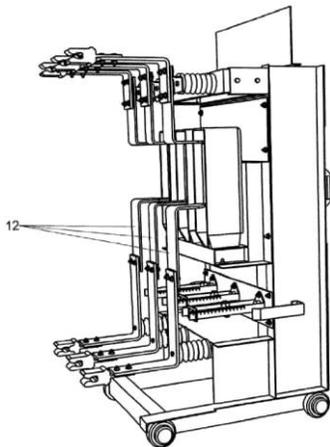
Fig. 3. Cubicle switchboard with the proposed measuring device (isometric view)
