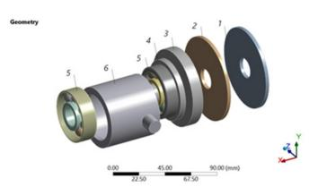
Figure 3: Nodes of multi-blade rotary friction tool: 1-heating cupped cutter, 2 - cutting cupped cutter, 3-sleeve, 4-shaft, 5-radial thrust bearing, 6-shell
