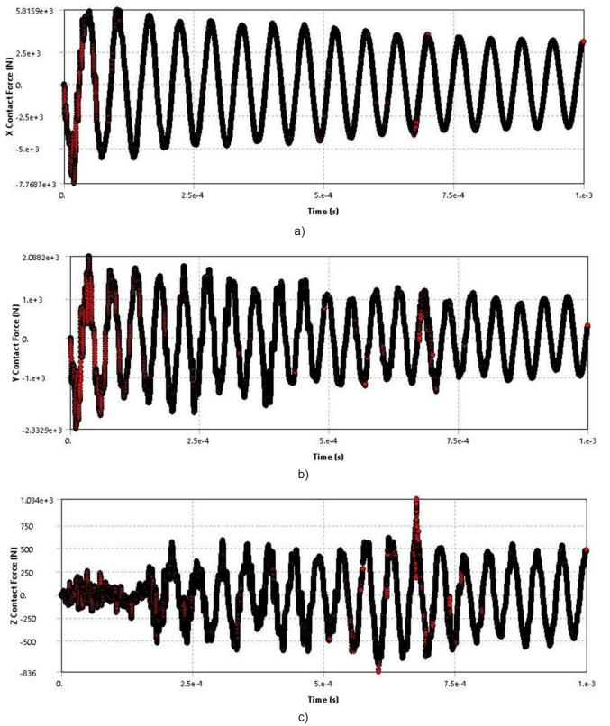
Figure 4: Predicted change in the projection of the cutting force of the cutting Cupped cutter: (a) X-axis; (b) Y-axis; (c) Z-axis
