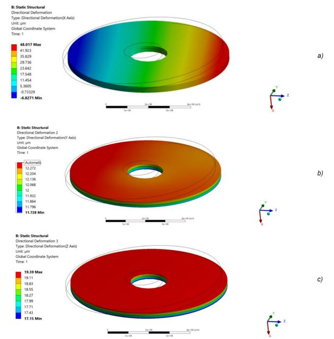
*Figure 10: The deformation picture in directions:a) along the X-axis;b) along the Y-axis;c) along the Z-axis*
