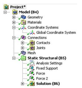
Figure 5: The project tree of the Static Structural module
