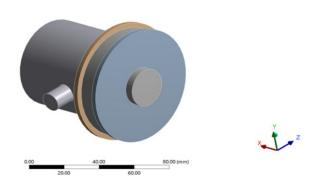
Figure 2: Three-Dimensional model of the body of a multi-blade rotary friction tool
