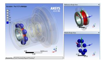
Figure 6: Setting up the bearing unit connection
