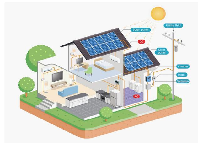
Figure 1 – A residential solar photovoltaic system
