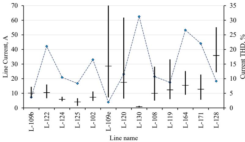
Fig. 10. Current harmonic distortion levels in the 110 kV electrical network of the West
