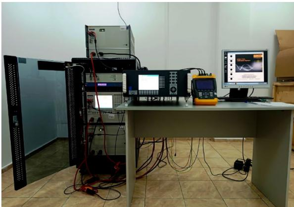
Fig. 1. Calibration process of the power quality analyzer in the Laboratory of Electric Power and Energy at the Republic of Kazakhstan Institute of Standardization and Metrology
