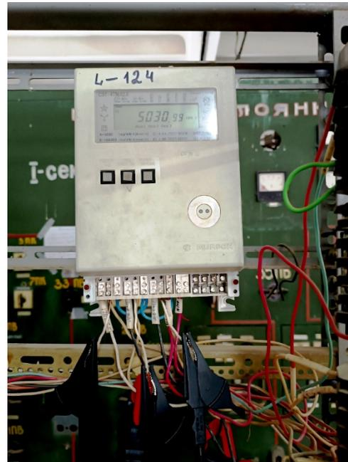
Fig. 2. Measurement of operating parameter connection of three-phase power quality analyzers to «L-124»
