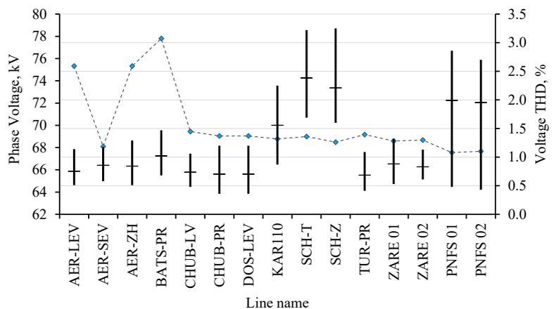
Fig. 5. Voltage harmonic distortion levels in the 110 kV electrical network of Astana
