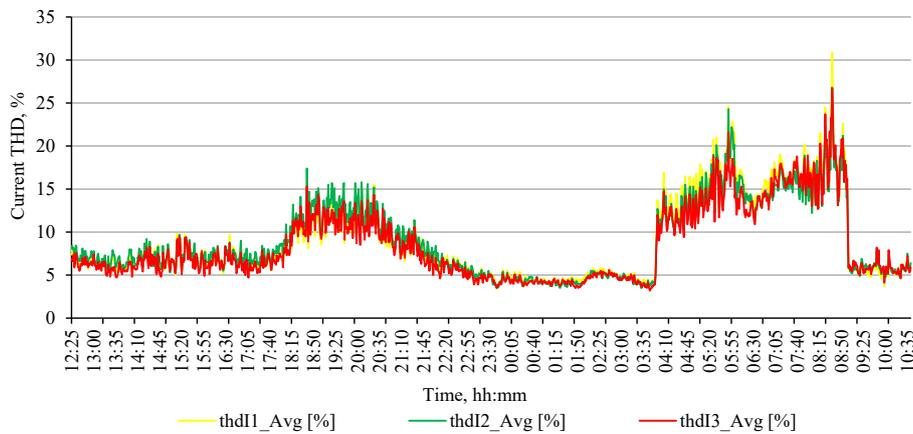
Fig. 3. Daily plot of current total harmonic distortion in one of the investigated 110 kV lines
