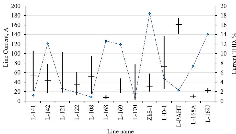
Fig. 8. Current harmonic distortion levels in the 110 kV electrical network of the South
