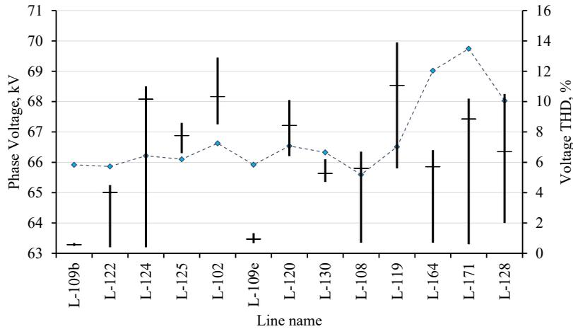
Fig. 9. Voltage harmonic distortion levels in the 110 kV electrical network of the West
