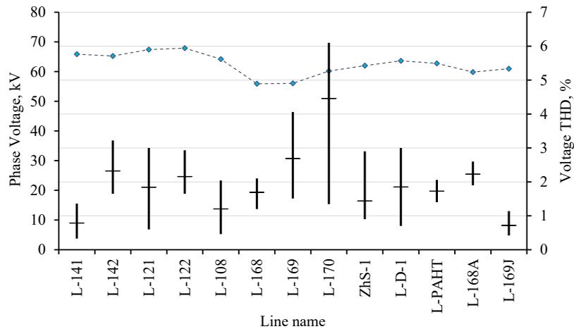
Fig. 7. Voltage harmonic distortion levels in the 110 kV electrical network of the South
