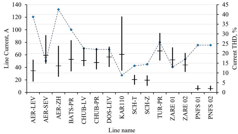
Fig. 6. Current harmonic distortion levels in the 110 kV electrical network of Astana
